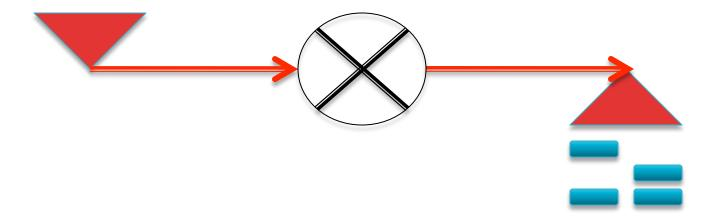
Some segments come out the other end; Sender uses timeouts to repair losses. Postel: only retransmit segment you know is lost!
